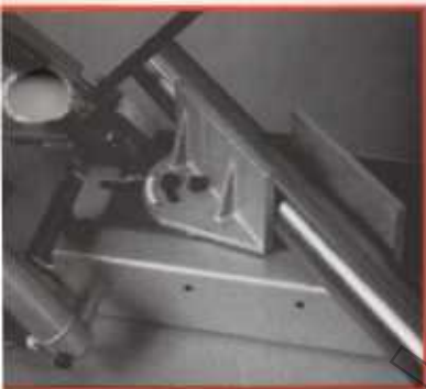
Blade guides (showing angle setting).
