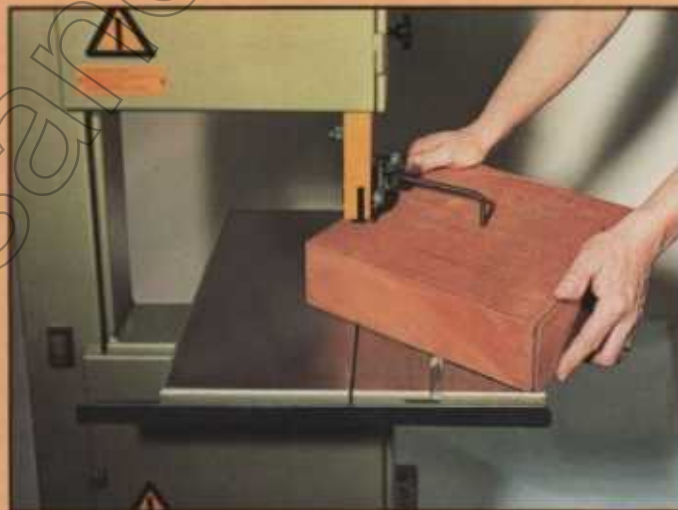
Circle cutting is simple using the standard circle cutting attachment.
