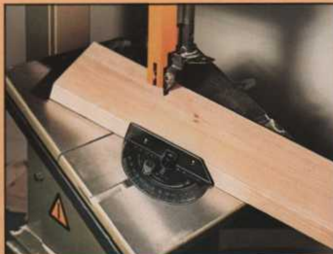
Tilting table and mitre guide allow compound angle cutting.
